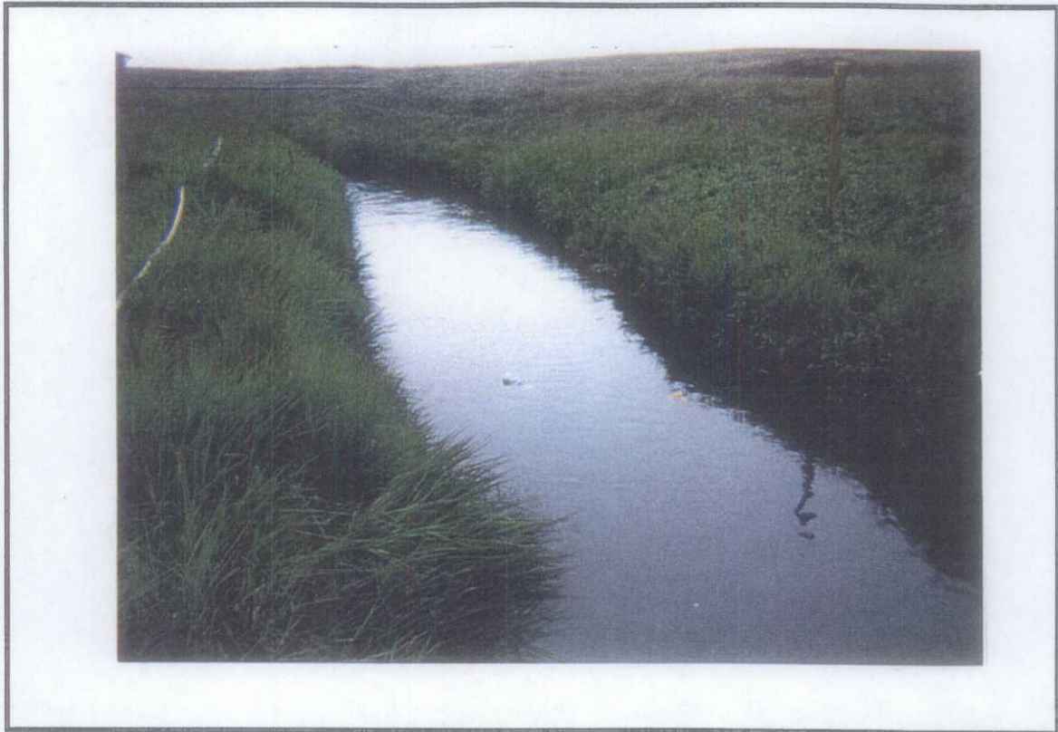
Stream Flow Measurement #8, Near Bridge at Site #2 Note Flotilla - used to time flow avg. of three clockings
