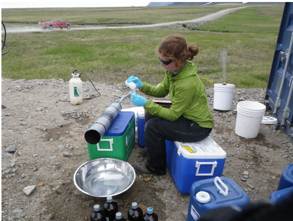
Photograph 9: Collecting rinsate sample from modified clam gun and stainless steel bowl. Direction: N/A. Date: July 2012.
