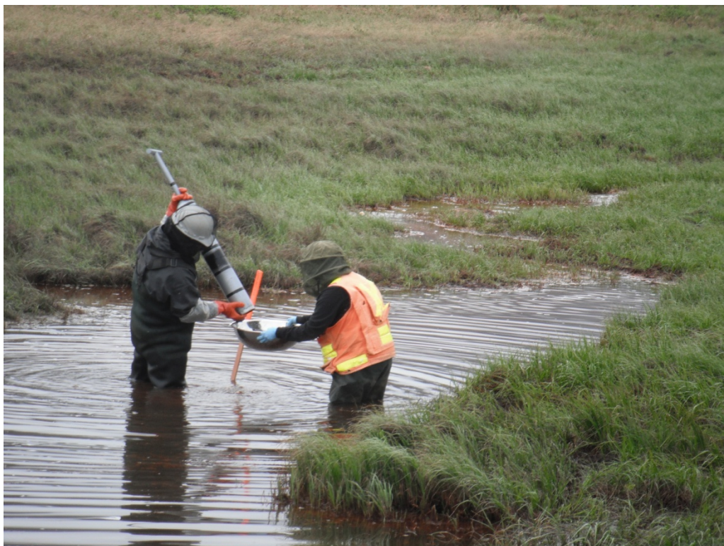
Photograph 5: Collecting sediment sample 12NC28SS023 using the modified clam gun. Direction: South-Southeast. Date: July 2012.
