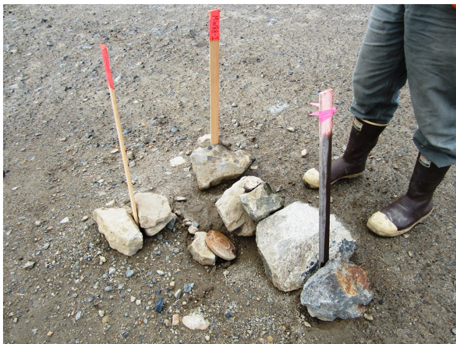
Photo No. 72 – 15 September 2013 Existing non-secured, frost-jacked monitoring well at Site 19. View facing north.
