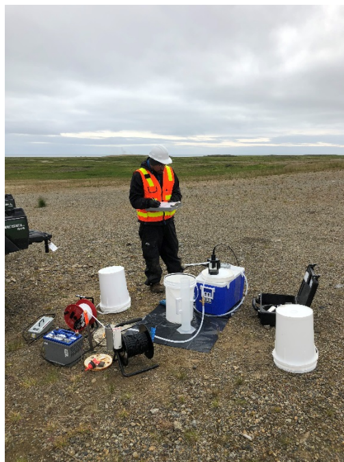
Photo No. 15 – 04 August 2018 Purging groundwater at Monitoring Well 88-1. View facing north.
