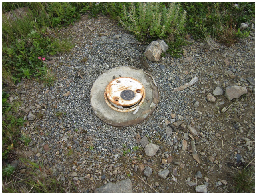
Photo No. 14 – 02 August 2018 View of monitoring well 17MW1 affected by frost-jacking. View facing down.
