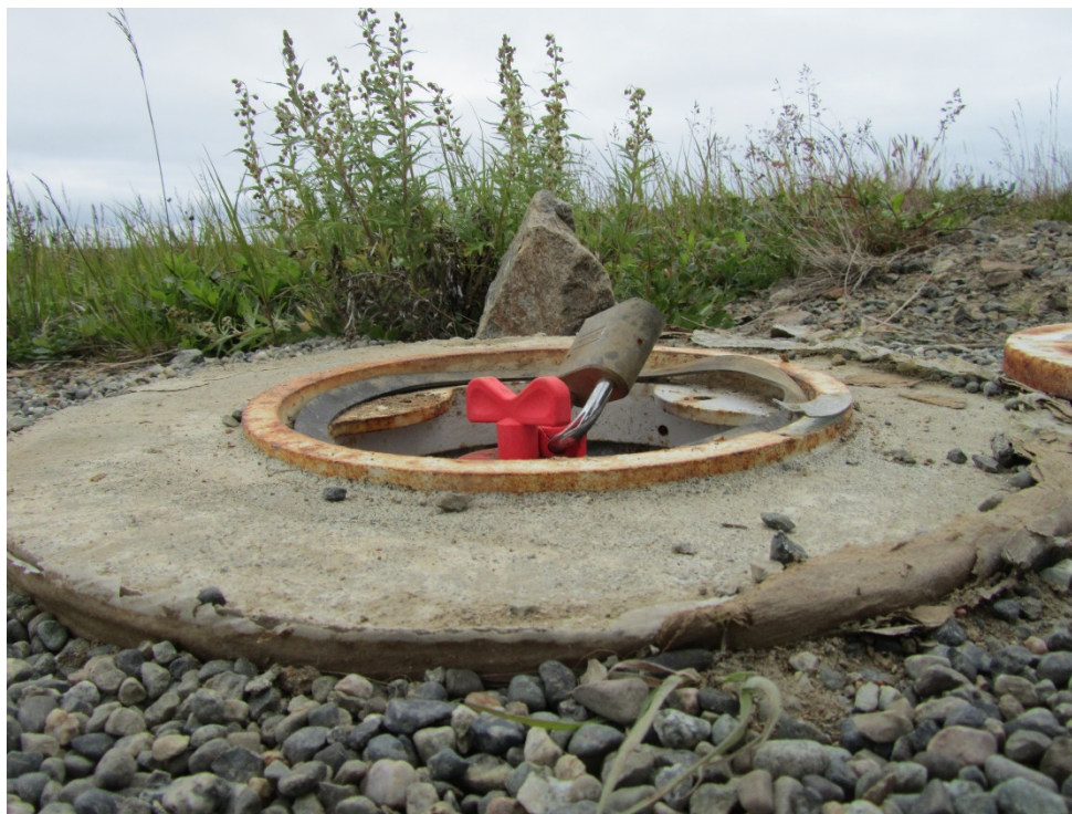
Photo No. 31 – 04 August 2018 View facing north of frost-jacked well 14MW05
