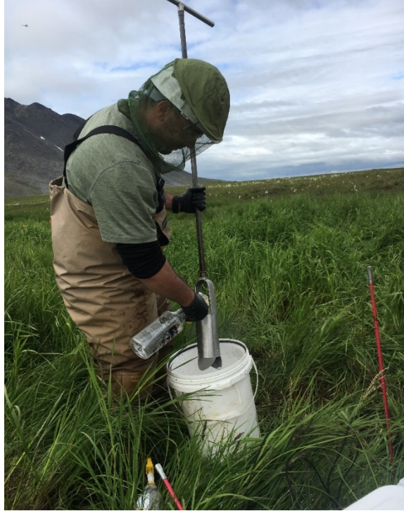
Photograph F-3-7: Decontaminating sample collection equipment during sediment sampling at Site 28. View facing west.
