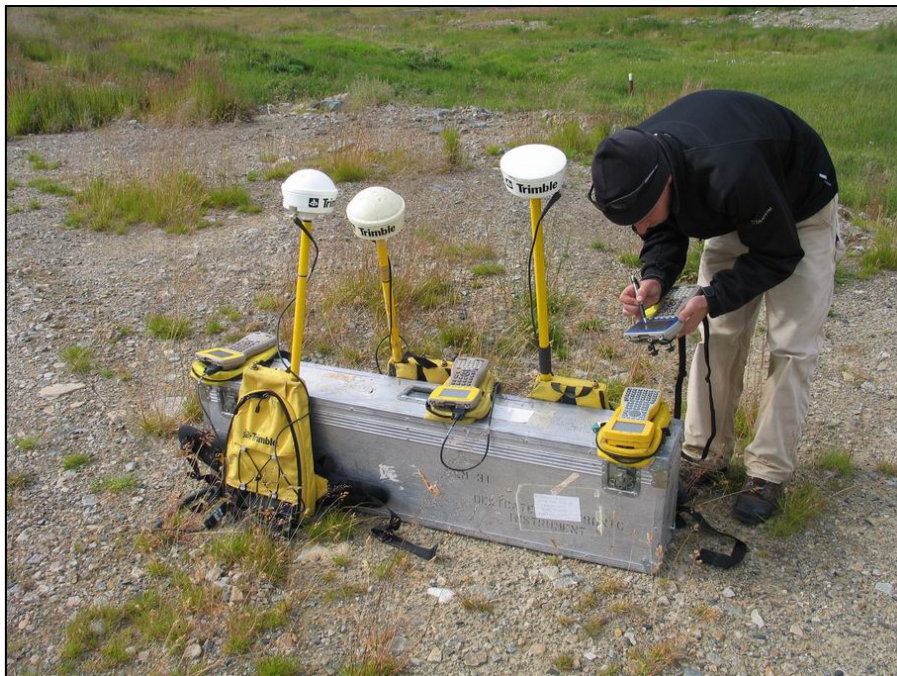
Performing time calibration of geophysical data loggers to GPS. (8 August 2007)
