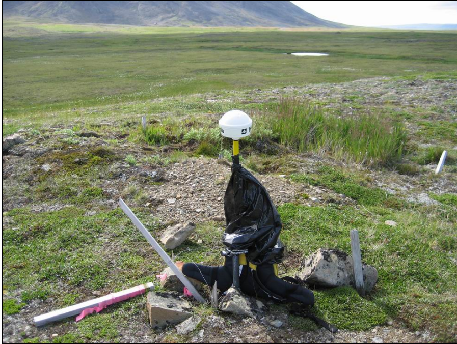
GPS base station set up on Benchmark BM-B 1951. (10 August 2007)
