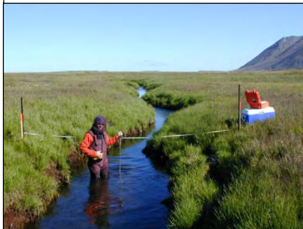
Photo (2002). Measuring streamflow in the Suqitughneq River downgradient of the Drainage Basin/Main Complex.
