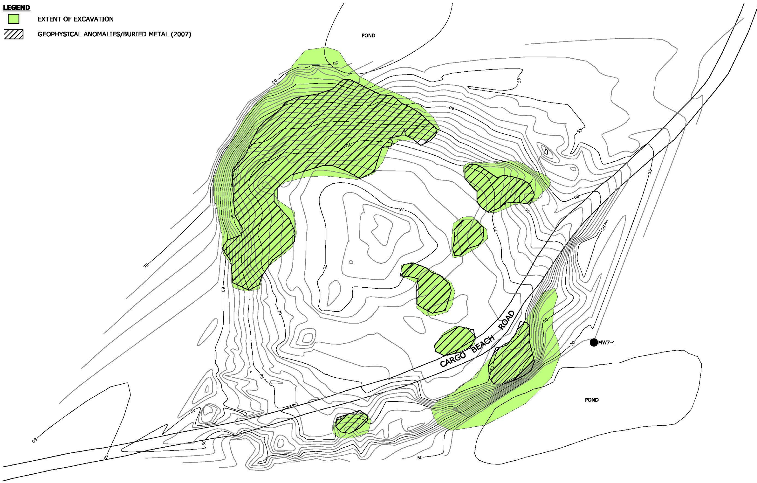
FIGURE 4 NORTHEAST CAPE, ST. LAWRENCE ISLAND, ALASKA IN-SITU CHEMICAL OXIDATION AND INTRUSIVE DRUM REMOVAL/LANDFILL CAP EXTENT OF SITE 7 EXCAVATION
