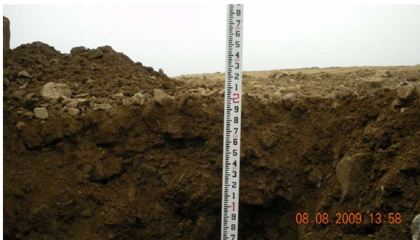
Photograph 6. Measurement showing a 2-foot-thick cap in a test pit in the landfill.
