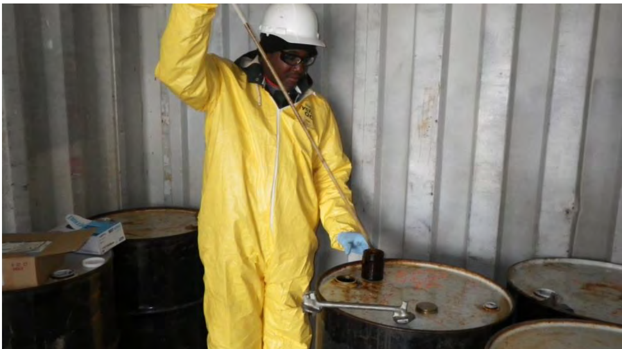
Photograph 52 Site 10, extracting drum samples with a drum thief. Direction: NA, interior of shipping container August 21, 2012
