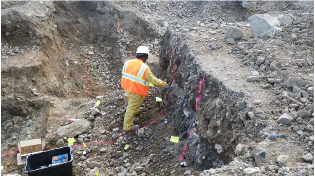
Photograph 39 Confirmation sampling for PCBs at Site 13. August 7, 2012
