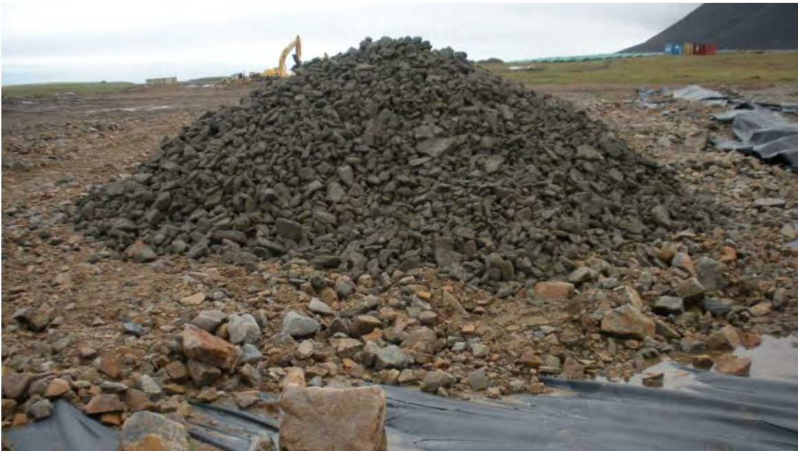
Photograph 26 Screened material from Pad 98. Material shown here was reject rock exceeding 2 inches in diameter. July 26, 2012
