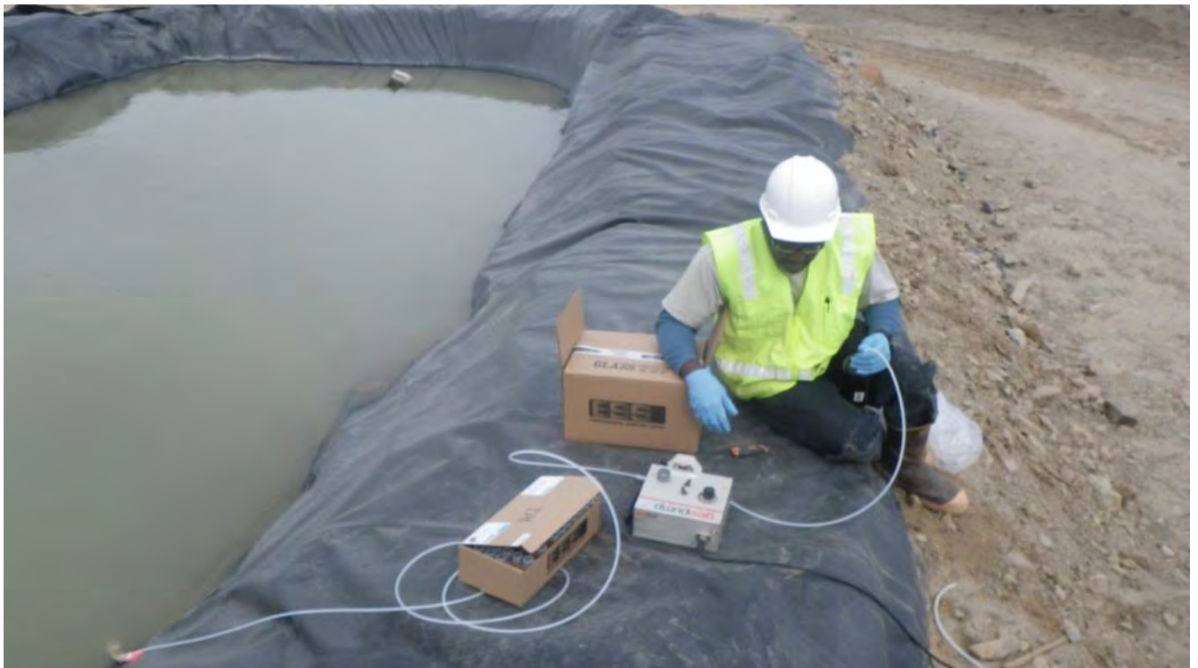
Photograph 44 Characterization sampling of MOC Impoundment water. August 12, 2012
