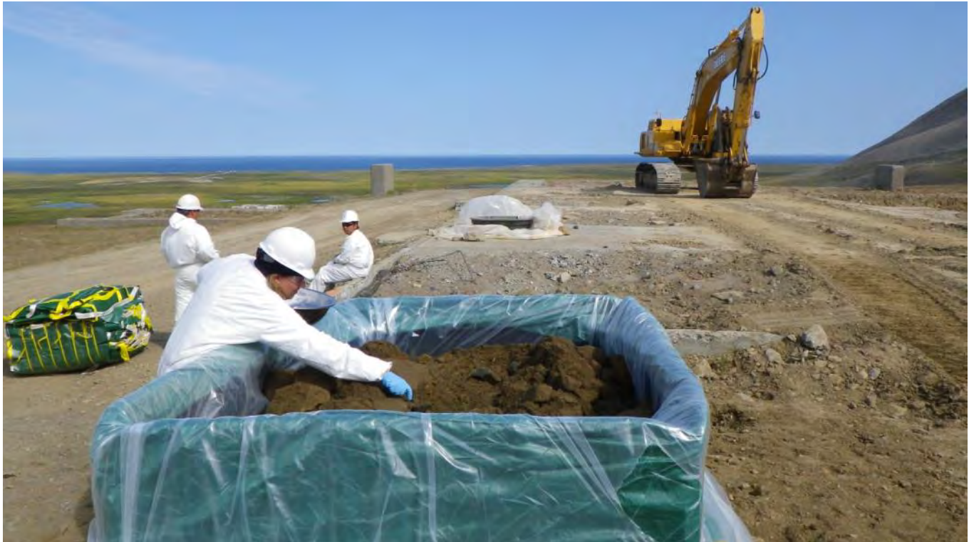
Photograph 43 Bulk waste characterization sampling at Site 31. August 11, 2012
