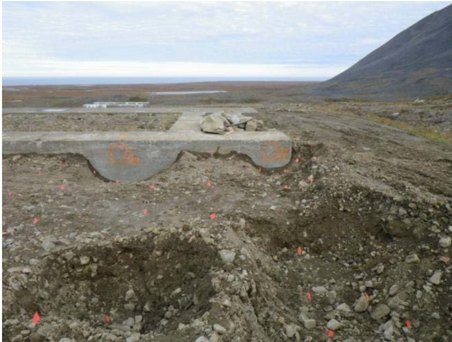
Photograph 47 Concrete wipe-sample locations 16 and 17 marked with orange marking paint September 16, 2011
