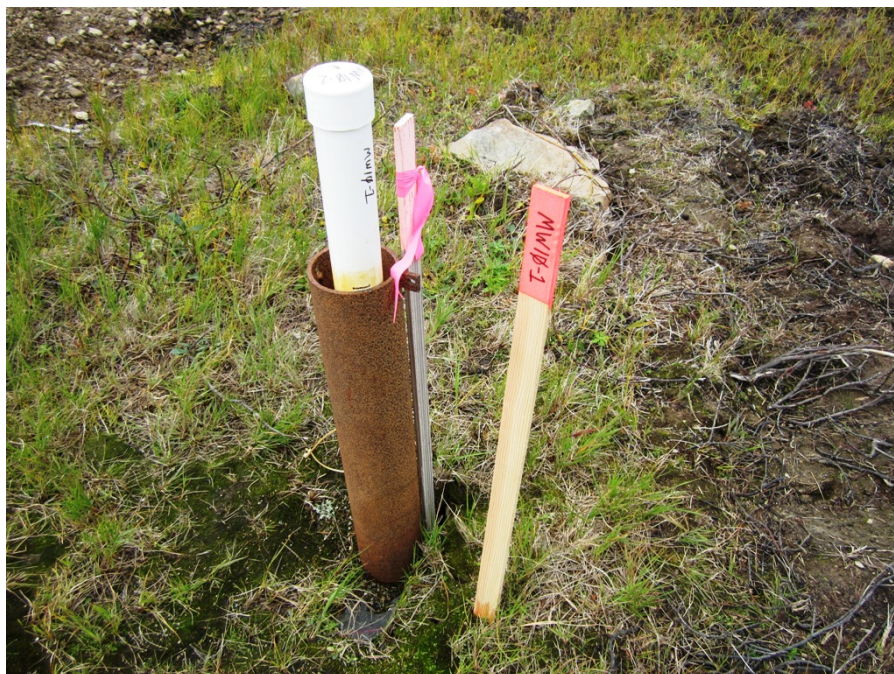
Photo No. 53 – 14 September 2013 Existing non-secured, frost-jacked monitoring well at Site 10.
