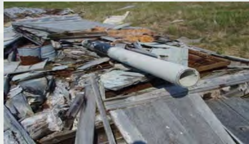
Debris and asbestos transite pipe
