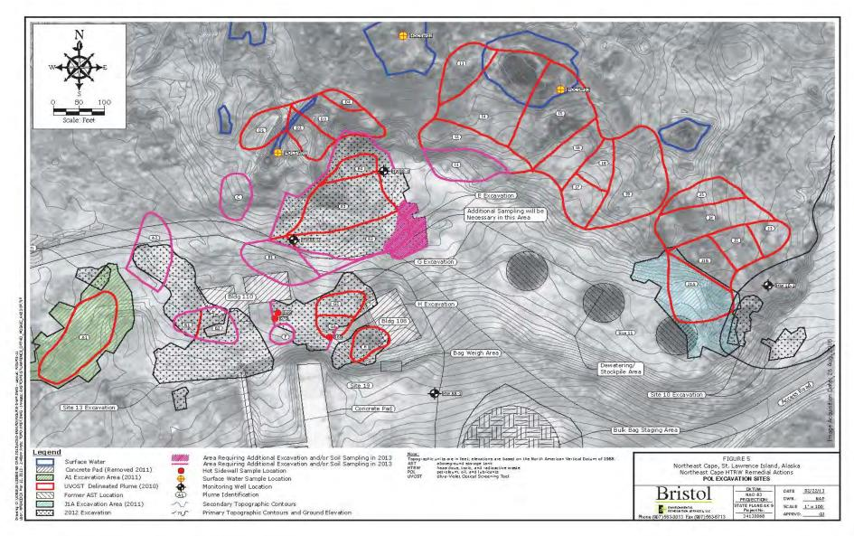
Excavation and disposal of PCB-contaminated soils from Site 13 (Heat and Power Plant) and Site 31 (White Alice Communications Station)
