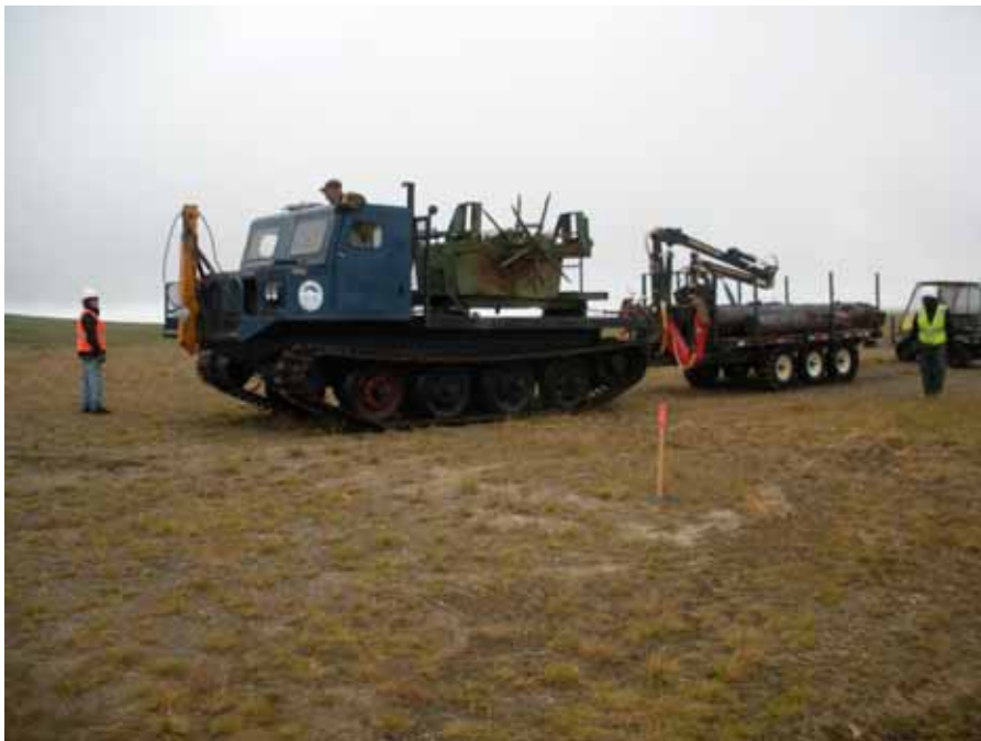
Photograph 46: Pole-pulling operation with Nodwell vehicle near MOC. Direction: west. Date: August 2010.
