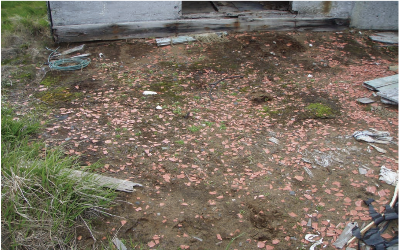
Photograph #17: Structure #5 ACM Suspect Broken Tile Direction: South
