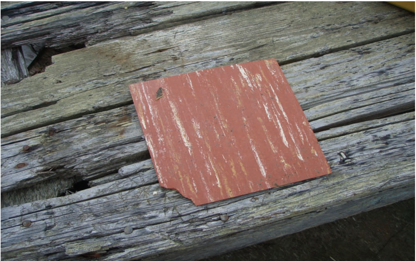
Photograph #7: 9" x 9" ACM Tile Outside Structure #3 Direction: N/A
