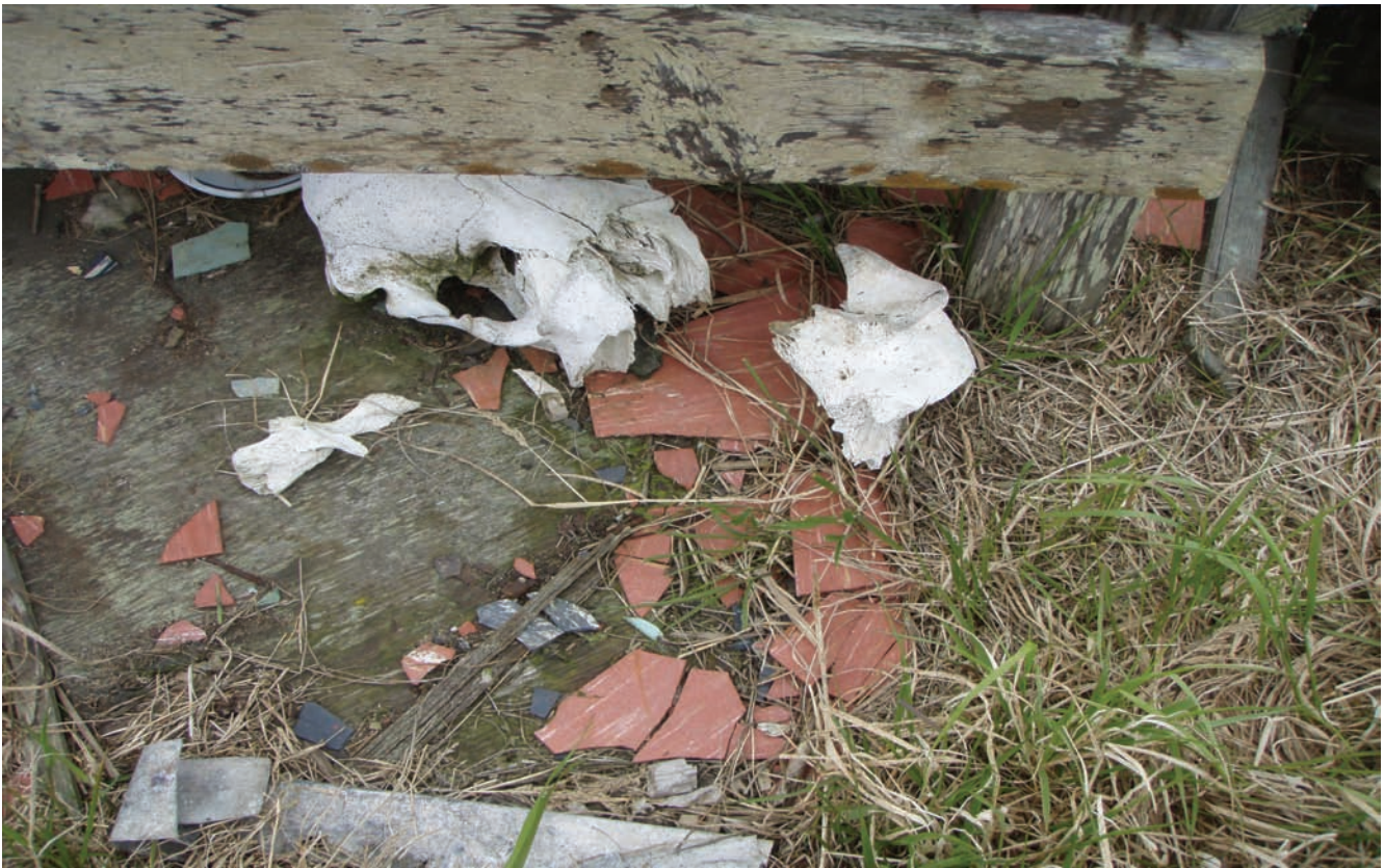
Photograph #9: Broken 9' x 9' ACM Tile Outside Structure #3 Direction: N/A
