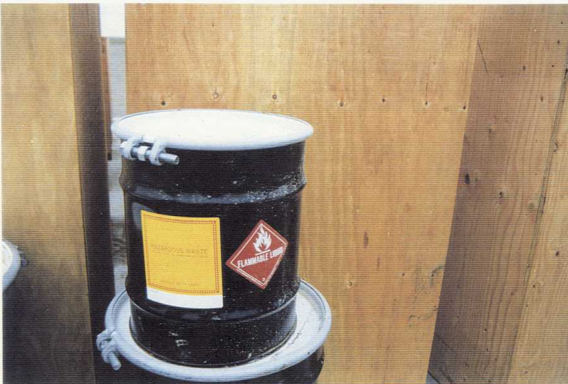
Fig. 3.36 Flammable wastes packaged, labelled and marked per USEPA and USDOT regulations. Viewed southerly at staging area at Northeast Cape on St. Lawrence Island, Alaska on 7/30/94 by Larry Wilkinson, Northwest EnviroService, Inc. on Contract DACA85-93-C-0048.
