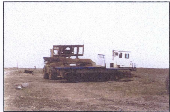
Photo 28: Loader placing runway matting on Nodwell.
