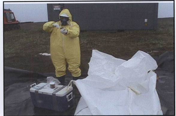
Photo 50: Sample collection to characterize soil in supersack at Site 8.
