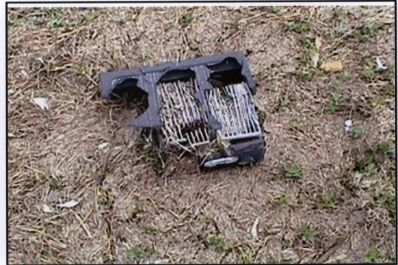
Photo 44: Deteriorated battery at Site 12.
