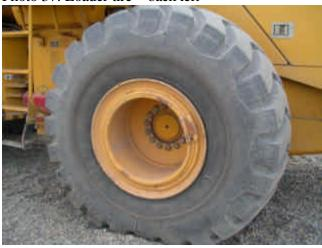
Photo 39: Loader with back tire needing air
